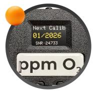
**RED (>100 ppm), ORANGE (30-100 ppm), GREEN (below 30 ppm)** At a glance, the unique colored LED strip shows the ppm value in the forming chamber. These values can be easily adjusted as desired. The signaling is also supported by an acoustic alert.
